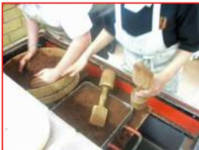
Forming the sand mould
