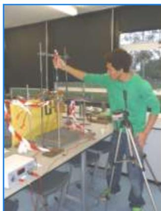
I am investigating how the angle of attack of a model swept wing affects lift. My challenge has been to determine a way to measure lift and I did this by seeing how the wings weight changes with an air flow over it. I found it useful to reaffirm theory with experiment.
